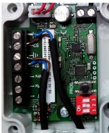
Illustration 31: Connecting the anti-crushing devices to the JCM transmitter RB3R868
