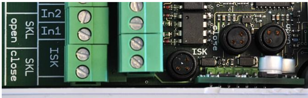
Illustration 22: Electrical connection of anti-crushing safety protection devices and ISK
